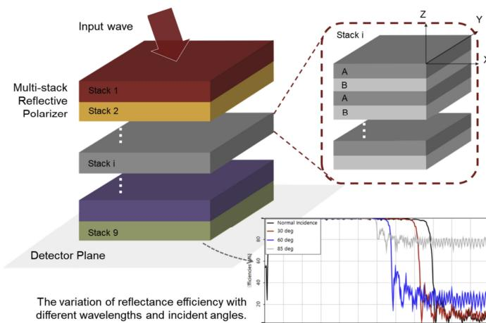
**NEW:** Stratified Media Component: Consists of stacks of alternate isotropic and anisotropic layers
