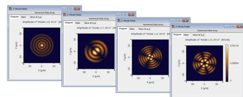
Fiber Mode Calculator to analyze LP Bessel
